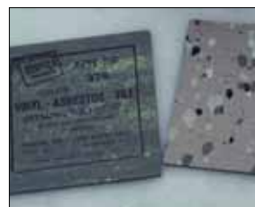
These asbestos cement pipes are labelled, so are the tiles, but you might not know until you start to lift them.
