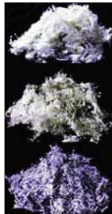
There are three 'colours' of asbestos, but you can't tell just by the colour what you have found; it could be mixed with other ingredients which change the appearance.
